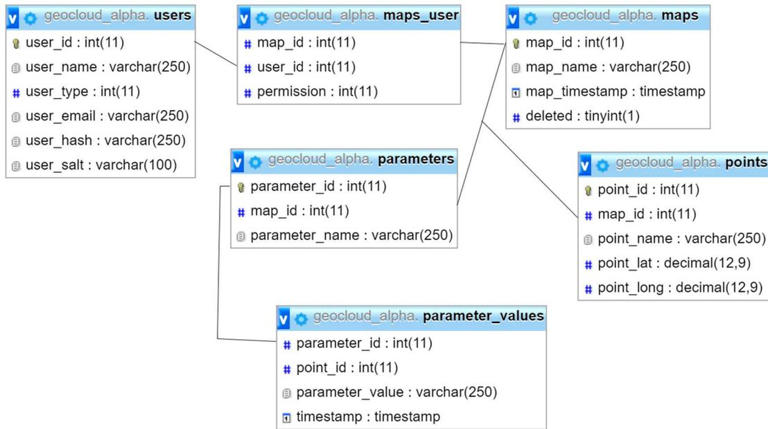
**Figure 3.** Diagram showing the relational database structure of the third development stage.
